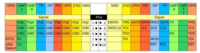
Table 1: Overview of target board pinouts in top view
